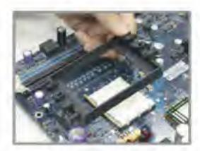
Turn to the back side of the motherboard and remove the back plate.
